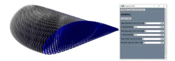
With WAM, you can effortlessly import any 3D design file and witness real-time magic unfold. WAM automatically calculates crucial parameters such as tape positions, tape lengths, tape angles, final build weight and material requirements, simplifying cost calculations.
